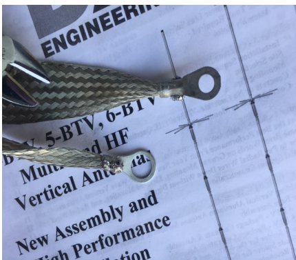
Stranded braid used to ground the antenna, mast, and tilt over base to the pool cage.
