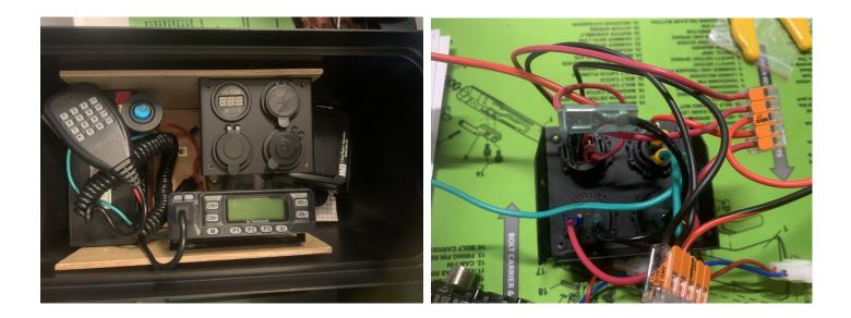
This is the old VHF/UFH setup in a plastic ammo can. This was my first rough attempt and took a long time as I didn't understand the correct way to connect the wires. It worked but was still a work in progress. This was followed by redoing the entire system and placing it in a metal ammo can which would also be a good ground plane for a mag mount antenna. The next picture is the new way of doing wiring using WAGO lever-lever nuts splicing connectors. These can be found on Amazon or at Lowes.
